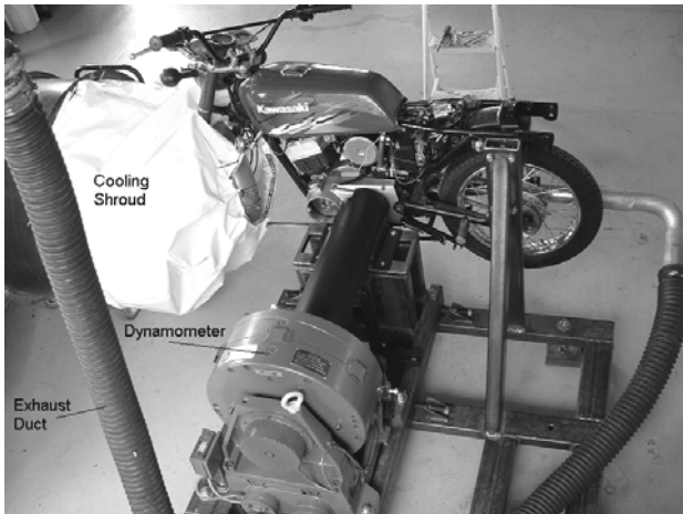
FIGURE 10 Motorcycle on the test stand. The dynamometer connects to the output sprocket. The cooling shroud directs air from a large fan for cooling.
