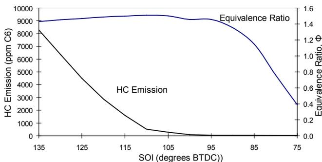
Figure 9 Trapped equivalence ratio and HC emissions versus SOI as predicted in a Wave computer simulation
