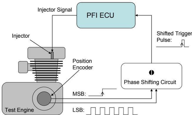
Figure 3 Schematic diagram of the injection shifting circuit
