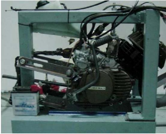
Figure 2 Engine coupled to dynamometer for testing
