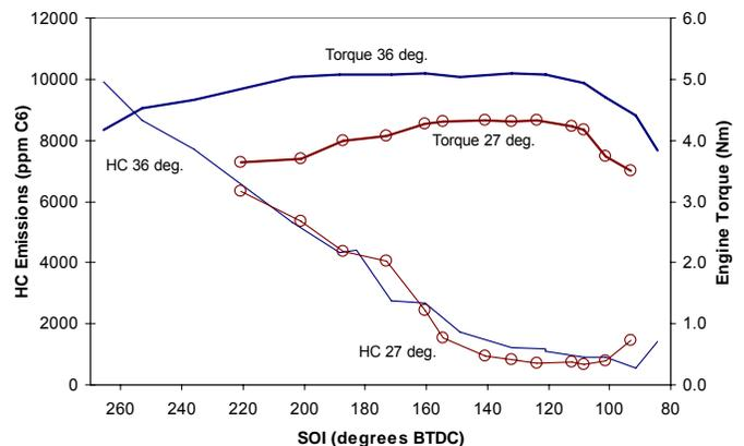
Figure 8 Torque (bold lines) and HC (fine lines) emissions as a function of Start of Injection timing for various injection durations.
