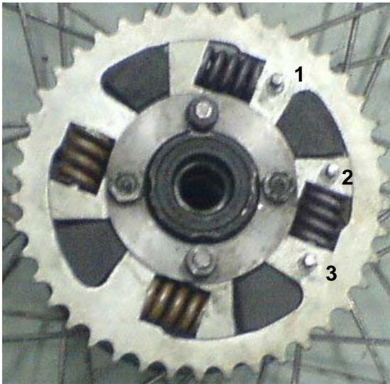
Figure 5 Special torque measuring sprocket used in the drive cycles studies
