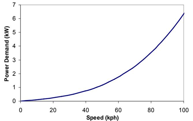
Figure 4 Engine power required as a function of steady state cruising speed
