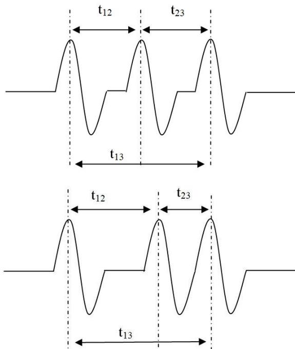
Figure 6 Signals from the torque measuring sprocket unloaded (top) and loaded (bottom)
